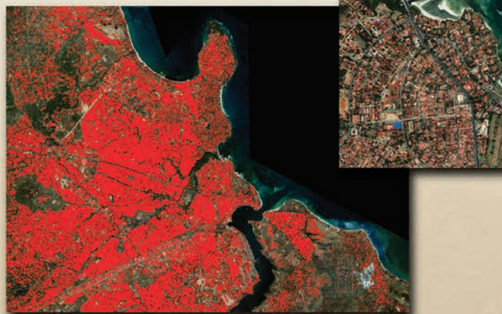
Dar es Salaam vector feature extraction: building footprints QuickBird imagery includes material Copyright © DigitalGlobe - Longmont, CO Vector Feature Extraction Courtesy of www.landinfo.com
